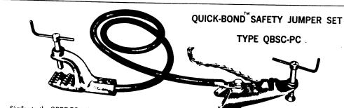
Similar to the QBPC-PC jumper set except that a Safe-C clamp is used in lieu of one Pipe Clamp. The Safe-C clamp attaches to structural shapes, plate, pipe wall or pipe (up to 2 in O.D.) Stainless steel speed screw breaks through tough oxides, paint, corrosion, etc., to make an excellent connection. Diamond studded jaw for excellent gripping and high psi contact.
