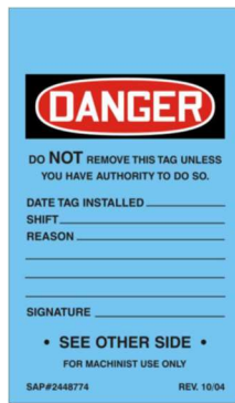
Tag used by Machinist to show isolation
