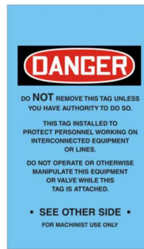
Tag used by Machinist to show isolation
