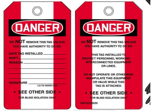
LOTO Rover's tag to verify isolation points
