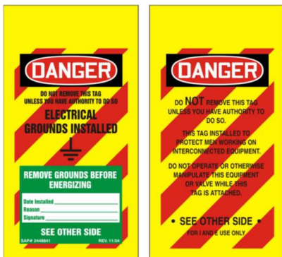
Tag used only by I&E indicating electrical grounds installed
